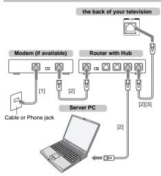
[1] Coaxial or telephone cable (depending on your modern type)[2] Standard LAN cable
